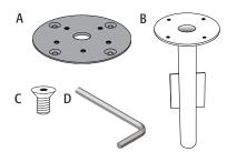
**STEP 1 Preparation**The in-ground fitting should or can be built into newly poured concrete. For a perfect flush mount, set the plate of the fitting 3/8" below the final surface grade. When you add the 3/8" thick adapter plate to the fitting plate, the adapter plate will be flush with the concrete.
