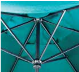
ARMS/RIBS The Portofino arms are 3/4" x 1-3/8" non-tapered and are secured to the ribs with stainless steel nuts and bolts.
