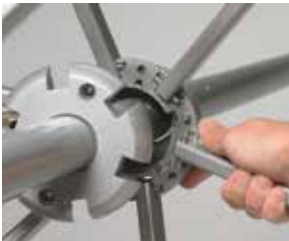
PORTOFINO II HUB The hub is cast aluminum and engineered for extra strength. It is split horizontally to encapsulate the stainless steel direct connect pin assembly. Two screws secure the hub together.
