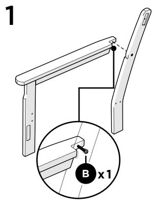
and align with pilot hole in the arm Duplicate other side
