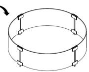
WARNING: ALLOW GLASS TO COOL BEFORE TOUCHING. IF PICKING UP THE GLASS GUARD TO MOVE FOR ANY REASON, GRIP THE MIDDLE OF TWO OPPOSITE GLASS PANELS AND APPLY CONSTANT PRESSURE TOWARDS THE INSIDE OF THE GLASS GUARD.
