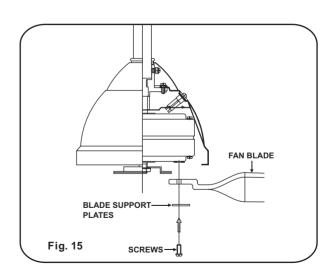
**Step 1.** Remove 1 of 3 screws from the motor housing and loosen the other 2 screws. (Do not remove)
