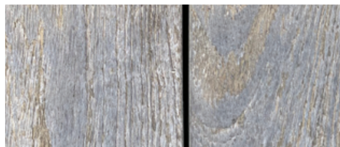
Advanced weathering (most finish worn away)
