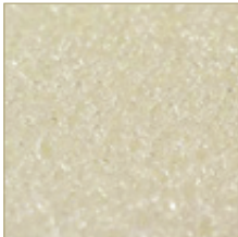
Reticulated Foam Highly porous 'flow-through' foam offers improved drainage over polyurethane foam while having less elasticity and a firmer sit.
