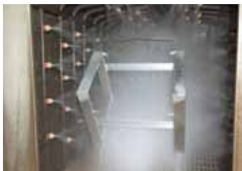
STAGE 5: CHEMICAL ETCH Seals and creates paintable surface.
