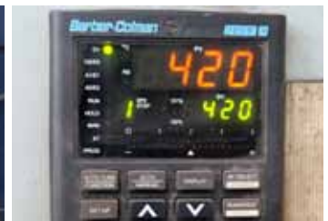
STAGE 8: PAINT CURE Powder-coat cures at an oven temp of 420 degrees for 22 minutes.
