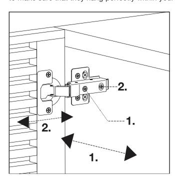
Use the **Phillips Screwdriver (A)** supplied to adjust Corridor's door hinges:
