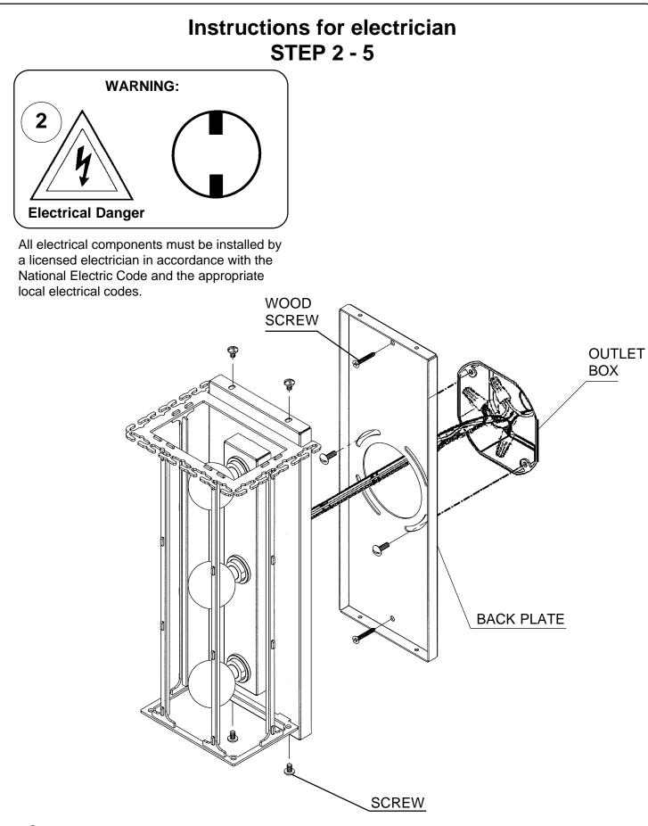
**3** Remove the (4) wall sconce screws and separate the back plate from the wall sconce. Feed stem and ground wires through back plate, then attach to power wires and ground wire in outlet box.
