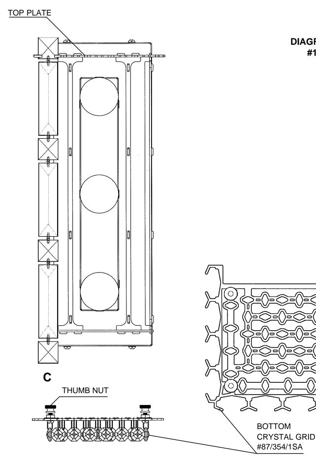
7 Install bottom crystal grid with four thumb nuts (already screwed onto grid) to bottom of the wall sconce.
