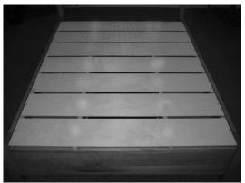
Attach the 5 remaining plywood deck pieces across the top of the unit using the remaining #10 x 1  $\frac{1}{2}$ " screws. Note the center deck piece has 2 sets of holes side-by-side. (See image above)
