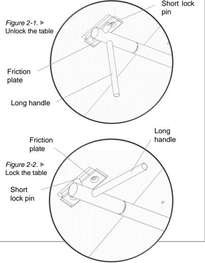
To lock the table, rotate the long handle on the lock mechanism till the short lock pin engages with the friction plate (*Figure 2-2*).
