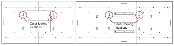
Figure 1-1. Outer locking position when leaf folded
