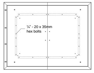
Figure 5. Insert 35mm hex bolts in 28 remaining locations
