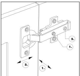
Use the **Phillips Screwdriver (A)** supplied to adjust Corridor's door hinges:
