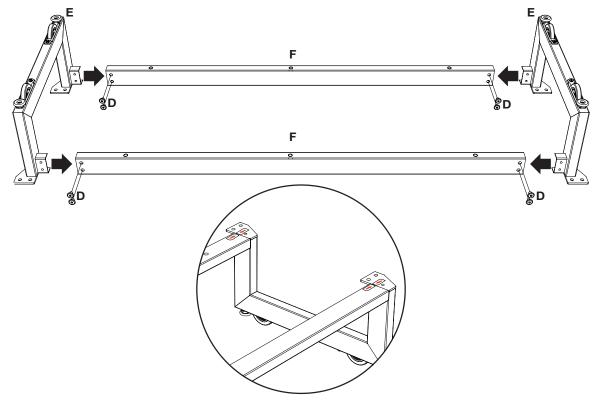
**Step 3 -** Carefully lay **Cabinet C** on its back. Using **Hex Wrench B1**, attach the base assembly to the bottom of the **Cabinet C** with **Screw D** and **Screw G**. \*Note: Each of the metal legs has levelers that can be adjusted using the **Hex Wrench B2**.
